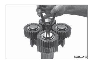
13 Pull off planetary gear.
