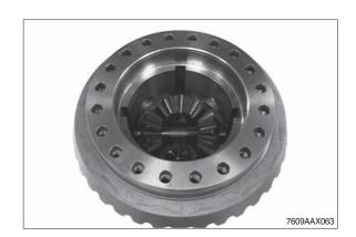
⑤ Remove the second axle bevel gear.
