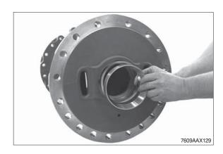
Mount two locating pins and bring the axle housing into contact position with the axle drive housing by means of the lifting device.
