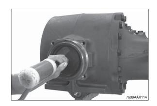
$\bigcirc$  Insert the determined shim e.g. s = 1.00 mm into the housing hole.
