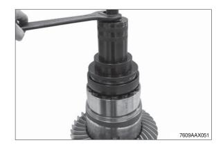
② Preload the differential by means of the press, loosen the hexagon screws and remove the releasing housing cover.
