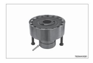
© Position the premounted differential with the lifting device onto the housing cover and preliminarily fix with hexagon screws.
