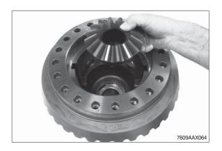
⑥ Lift the pressure ring out of the differential housing and remove the disk package and thrust washers behind.
