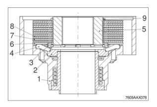
(3) Preload disk package with an axial force of  $F = 50^{+30}$  kN.
