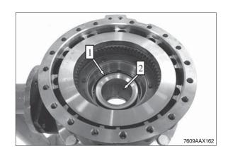
Align disk package centrally and radially.
