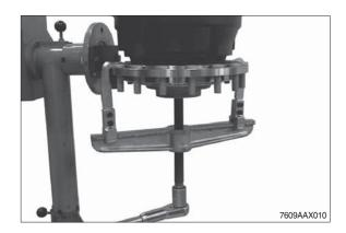
Lift the planetary carrier out of the brake housing by means of the lifting device.
