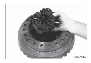
$\ensuremath{{\textup{7}}}$  Mount second axle bevel gear.
