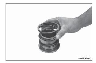
① Insert the premounted sliding sleeve into the housing cover.
