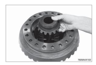
Insert the second pressure ring into the differential housing.
