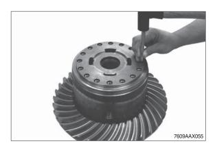
⑥ Force out both differential axles (short) and remove the releasing spider gears with thrust washers from the differential housing.
