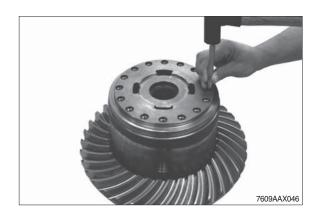
Force out both differential axles (short) and remove the releasing spider gears with thrust washers from the differential housing.
