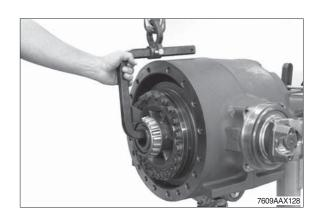
(8) Insert the determined shim (e.g. s = 1.1 mm) into the hole of the axle housing and adjust the bearing outer ring (see arrow) until contact is obtained.
