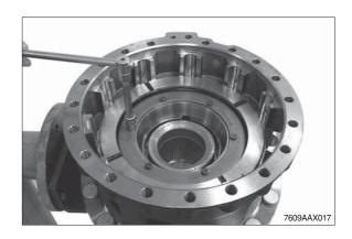
① Mount breather valve and press piston out of the brake housing by means of compressed air.
