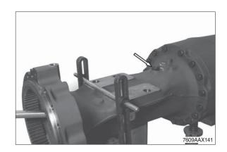
⑤ Provide screw plug with a new O-ring and fit it.
