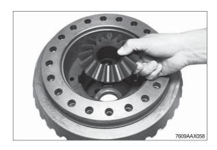
Press crown wheel from the differential carrier.
