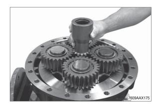
Fix determined shim (s) e.g. s = 1.60 mm with grease into the sun gear shaft.
