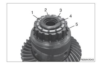
⑤ Preload differential by means of the press, loosen locking screws and housing cover.
