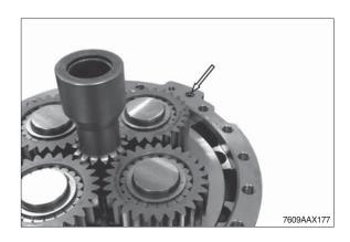
③ Grease O-ring (see arrow) and install it to the axle housing.
