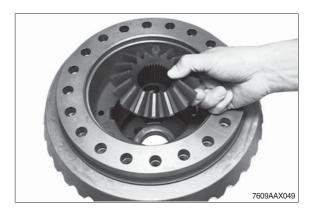
Press crown wheel from the differential carrier.
