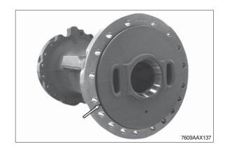
② Mount two locating pins and bring the axle housing into contact position with the axle drive housing by using the lifting device.
