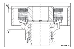
⑤ Position housing cover onto pressure piece (see arrow).
