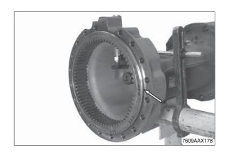
Mount two adjusting screws and use the lifting device to bring the output into contact position with the axle housing.
