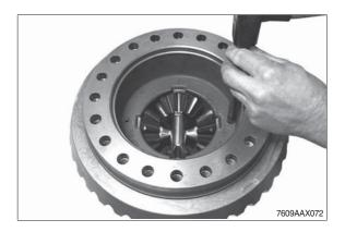
$\ensuremath{{\bigcirc}}$  Mount second axle bevel gear.
