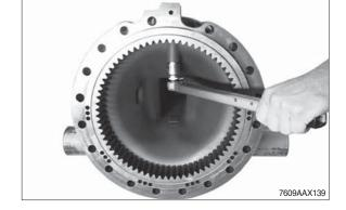
④ Grease O-ring and insert it into the annular groove of the brake tube (see arrow).
