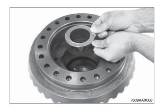
$\ensuremath{\mathfrak{I}}$  Insert axle bevel gear.
