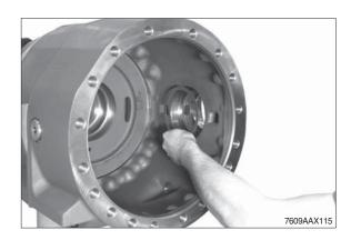
⑥ Undercool the internal bearing outer ring and bring it into contact position in the housing hole by using the assembly fixture.
