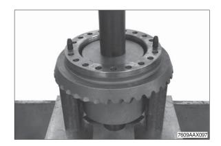
② Insert thrust washer into the differential housing.
