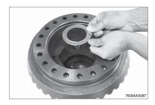
③ Insert axle bevel gear.
