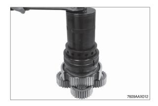
Disengage retaining ring.
