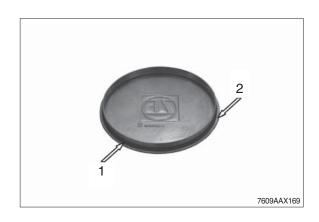
② Insert the cover into the output shaft until contact is obtained.
