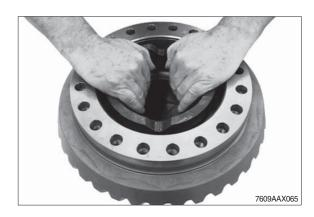
Press crown wheel from the differential carrier.
