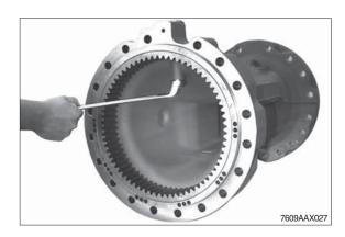
④ Pull the bearing outer ring out of the bearing hole and remove the shim behind.
