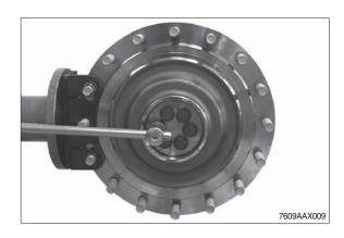
Press planetary carrier with a two-armed puller out of the profile of the output shaft.
