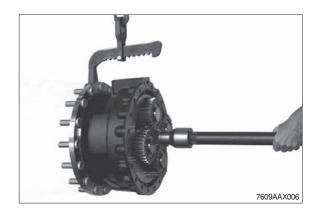
⑥ Fix output to assembly truck.
