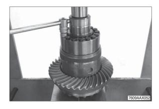
③ Preload the differential by means of the press, loosen locking screws and housing cover.
