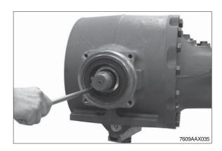
Press input pinion from the axle drive housing and remove the releasing tapered roller bearing.
